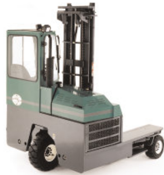
The low profile platform design ensures optimum stability and safer product handling
