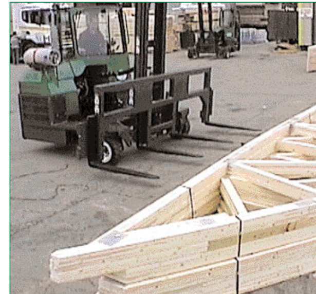
A 'quick-release' four-fork attachment is available for use with extra long loads.
