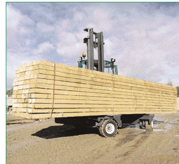
The Combilift is capable of working in un-paved yards and semi-rough terrain.
