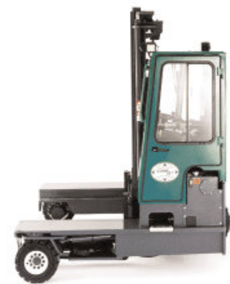
Machine with mast retracted enabling long loads to be rested securely on the platform.
