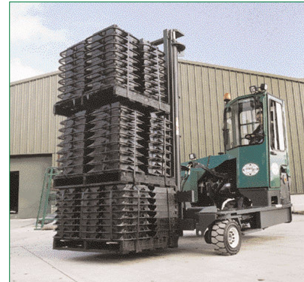
The Combilift can also work as a conventional counter balance forklift handling cube loads.
