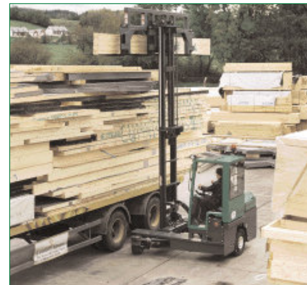
Space savings can be more than 50% in warehouses and yards, depending on the type of product stored and the existing aisle width.
